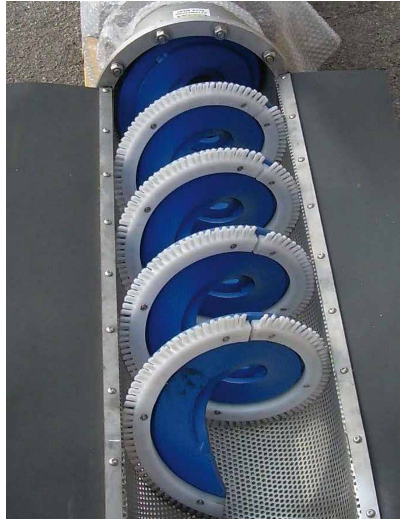
Brushes bolted and circular holes basket
