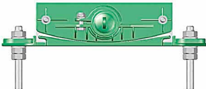
Fixed installations of strip diffusers with threaded rods.
